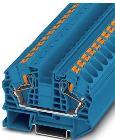
Feed-through terminal block, nom. voltage: 1000 V, nominal current: 76 A, connection method: Push-in connection, 1 level, Rated cross section: 16 mm<sup>2</sup>, cross section: 0.5 mm<sup>2</sup> - 25 mm<sup>2</sup>, mounting type: NS 35/7,5, NS 35/15, color: blue
